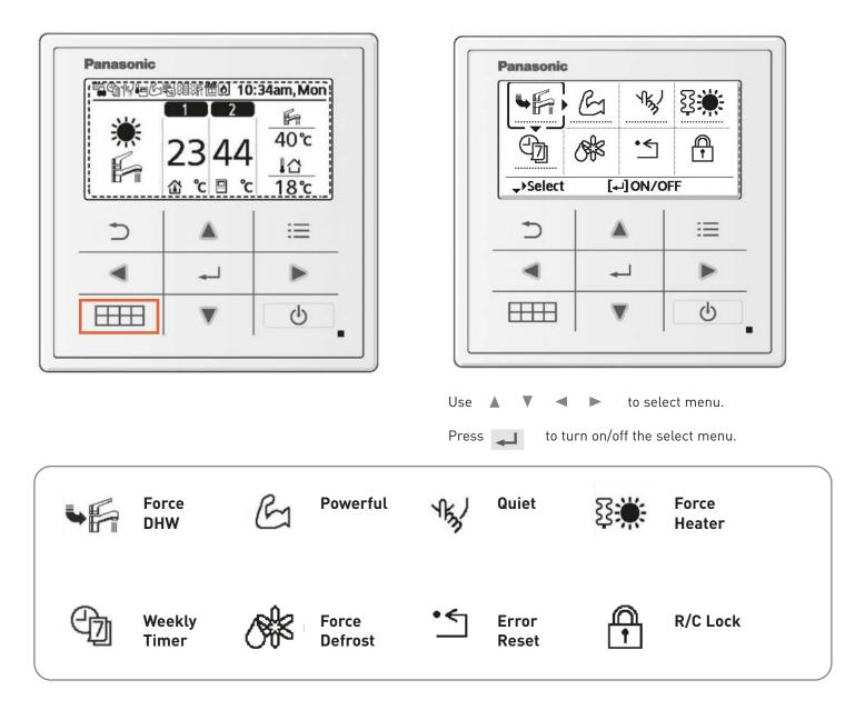
Select each setting and confirm the setting according to the instructions displayed at the bottom of the screen. (The icons refer to each selection key.)
