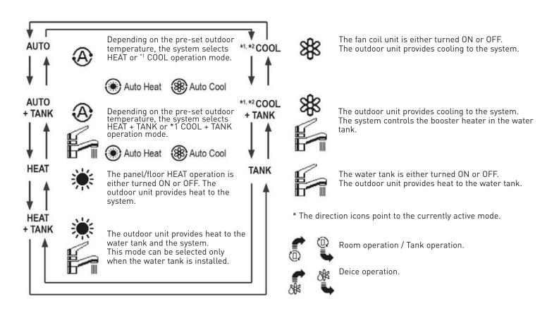
\*1 The system is locked to operate without COOL mode. It can be unlocked only by authorised installers or our authorised service partners. \*2 Only displayed when COOL mode is unlocked (This means when COOL mode is available).
